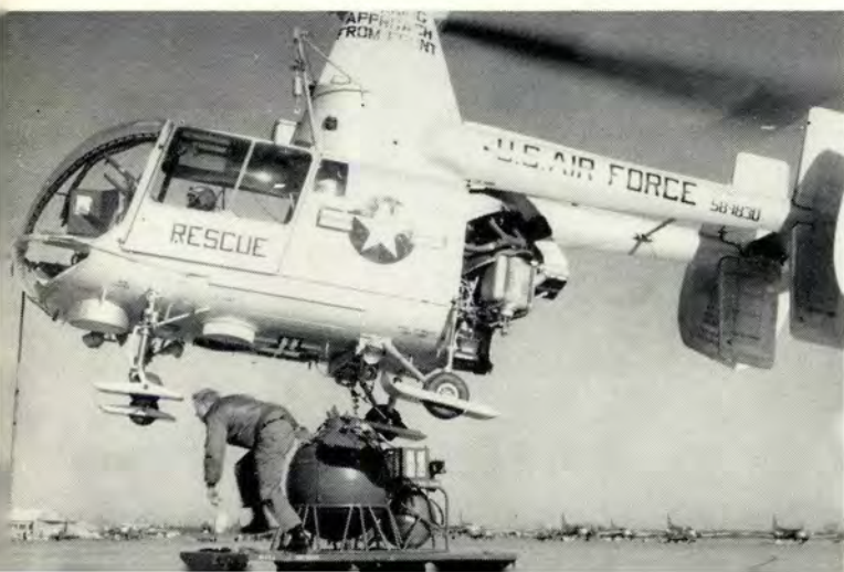
Above, the H-43 on alert and ready to scramble. Below, hooked up and ready. When ground crewman lowers positioning pole (in front of H-43), pilot is clear to go.
