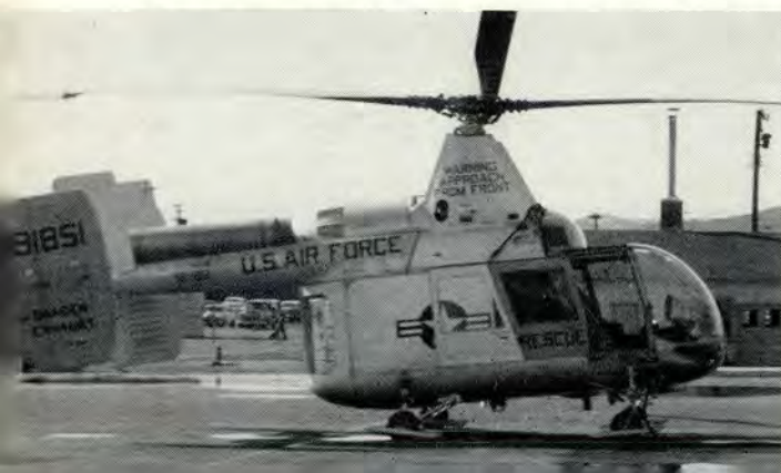
Above, A/IC Ray Owen, crew chief, shows hazard of rotor blades. The only safe place the aircraft can be approached from is the front. Below, the H-43B is shown for comparison. Note tailpipe on booms.
